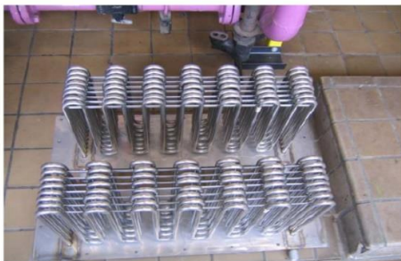
Figure 2-3: Photograph of Two Bare Tube Heat Exchanger Bundles.
